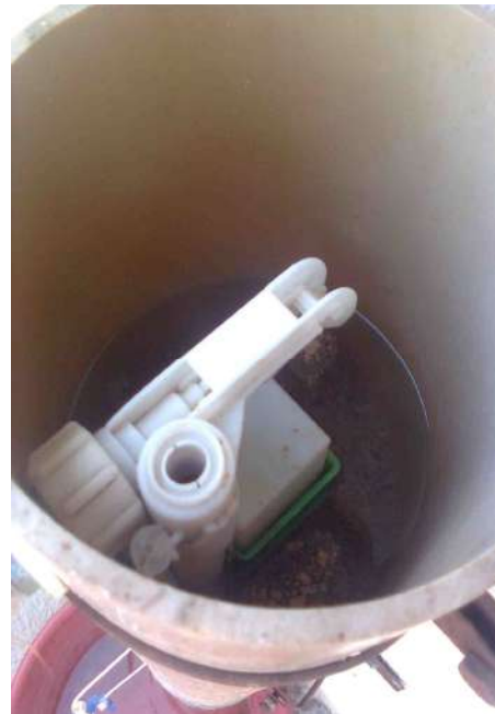
Figure 4.3: Mechanical float valve.
