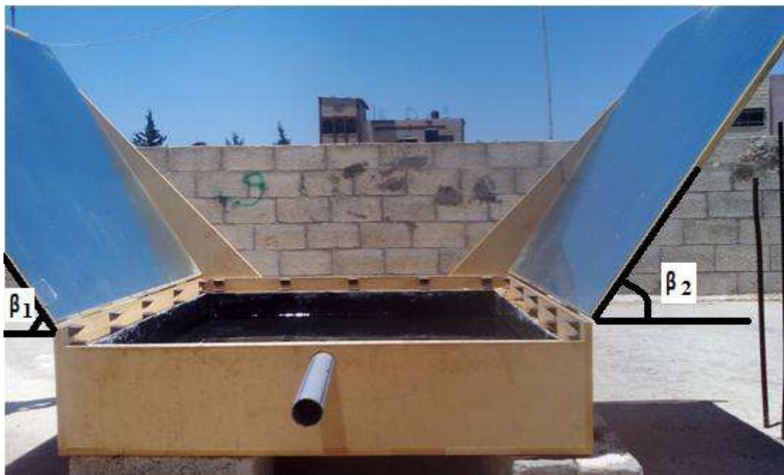
Figure 4.2: Photographic of Locally Fabricated SSP
