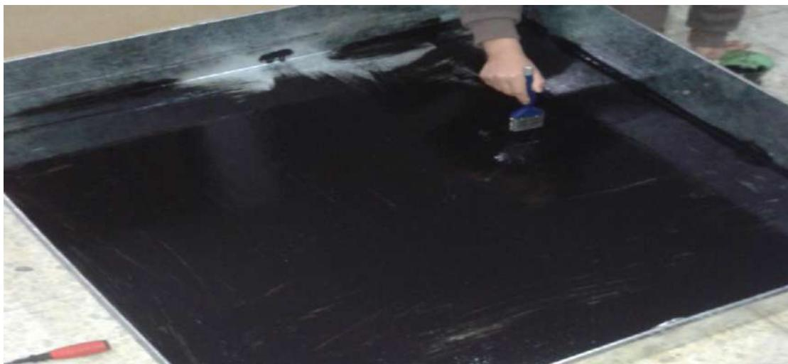
Figure 4.5 : The painting of absorber plate
