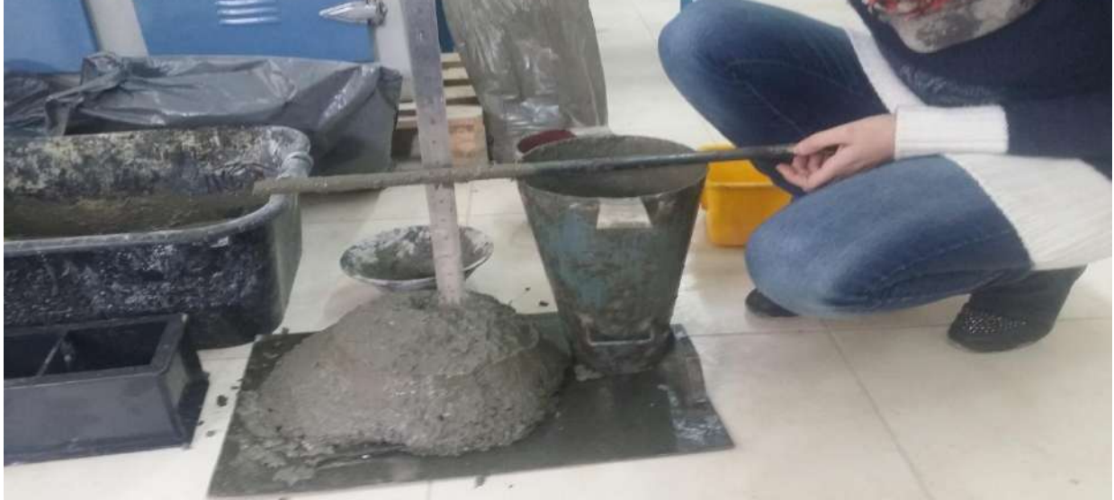
Figure 9: The mechanism of slump test of fresh concrete (measuring the reduction of fresh concrete mass)
