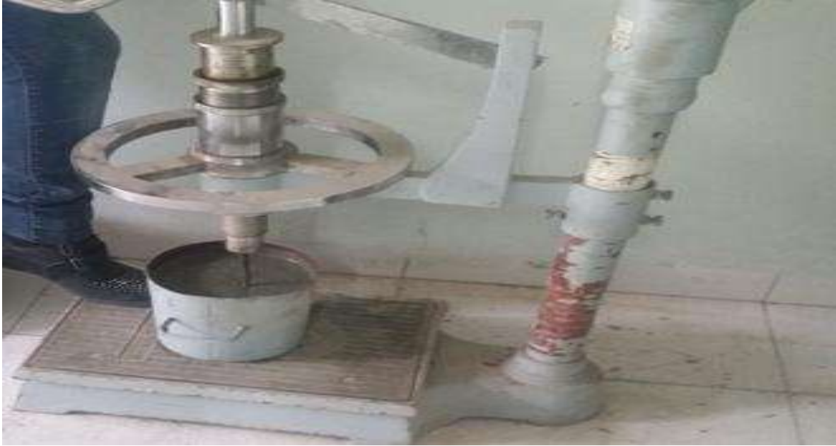
Figure 10: Concrete setting time test
